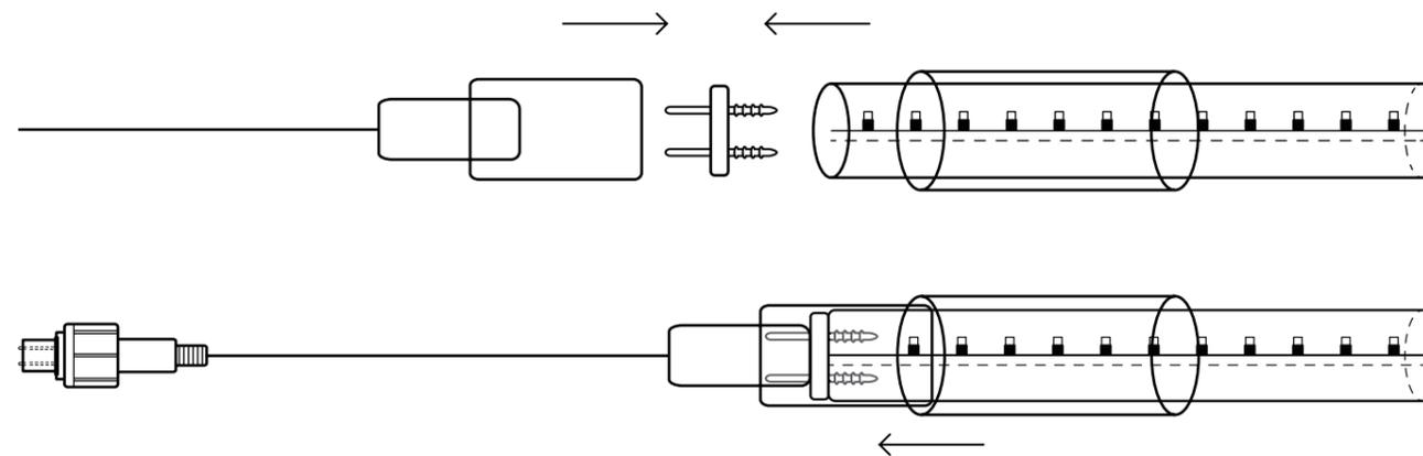
**4.** Move the transparent tube over connection and heat it using heat gun. Caution — it's hot!
