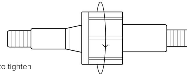
Twist the secure ring to tighten the plugs together.
